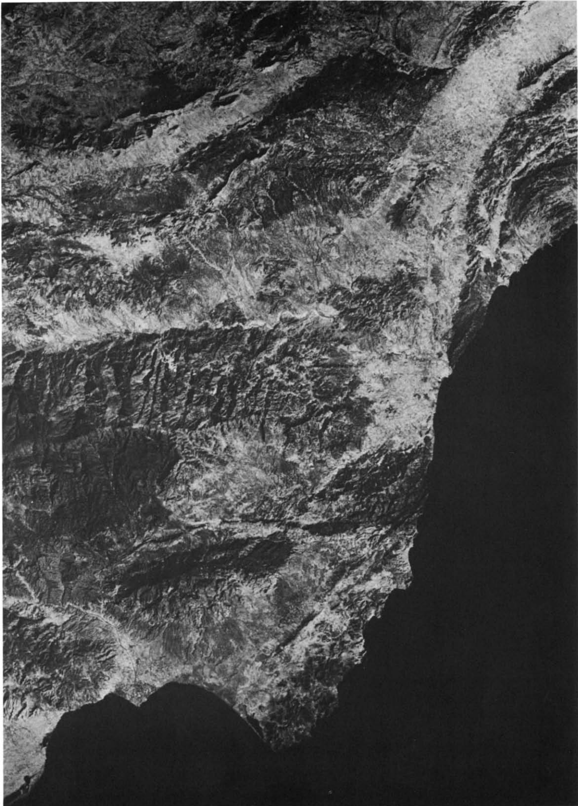
Fig. 4. Multispectral Scanner (MSS) scene of the area outlined in Fig. 3 made by the satellite Landsat 3 on 11th March, 1979, from 920 km height. Shown here are the band-7 data (near-infrared 0.8–1.1 \mu\text{m} wavelength). The scale of resolution is 79 m. The major structural features mapped independently on the ground and compiled in Fig. 3 are visible.
